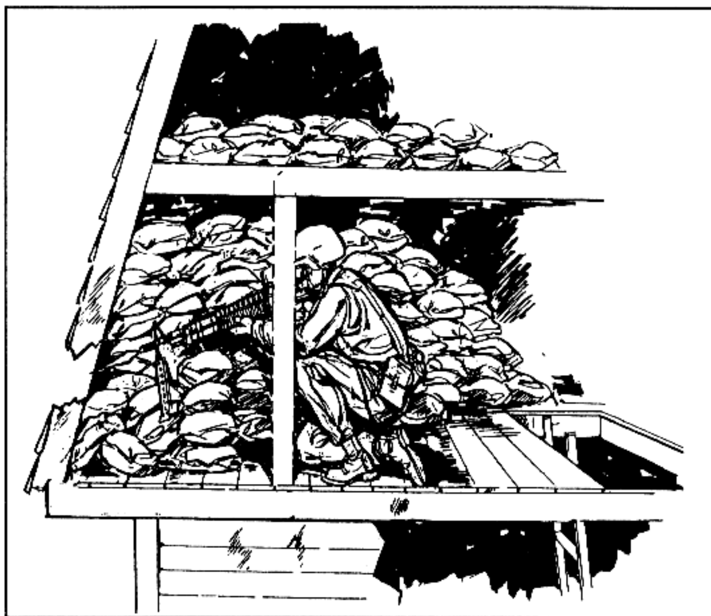
Figure 5-41. Firing platform built under roof.
